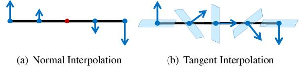
Figure 2: Obtaining continuous surface normals. The thick line is a surface of Minkowski sums and the surface normals with an opposite direction at both ends of the surface are annotated with blue arrows. (a) Surface normals are interpolated for the rest of the surface. However, the normal at the red point becomes singular. (b) Surface normals are obtained everywhere from tangent plane (blue) interpolation with no singularity.
