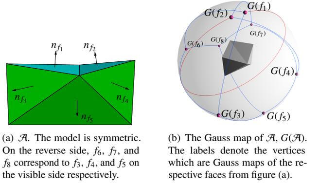
Figure 5: A non-convex polyhedron  $\mathcal{A}$  and its Gauss map,  $G(\mathcal{A})$ .
