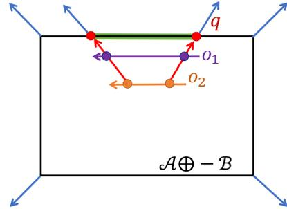
Figure 10: The purple and orange lines represent two moving origins  $\mathbf{o}_1$  and  $\mathbf{o}_2$ , respectively. Even though  $\mathbf{o}_2$  moves only slightly compared to  $\mathbf{o}_1$ , their Phong-projected results on the surface of the Minkowski sum occupies the same region (the green line). Thus, it is necessary to have an expanded search region for a deeply-penetrating configuration
