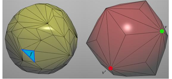
Figure 7: Convex maps are used to identify and repair convolution errors. The (blue) face  $f$  on the left convex map was compatible with the vertex  $v$  on the right before rotation. After rotation, our method finds  $f$ 's new associated vertex  $v'$  using gradient decent on the convolution of the convex maps (see details in Appendix).
