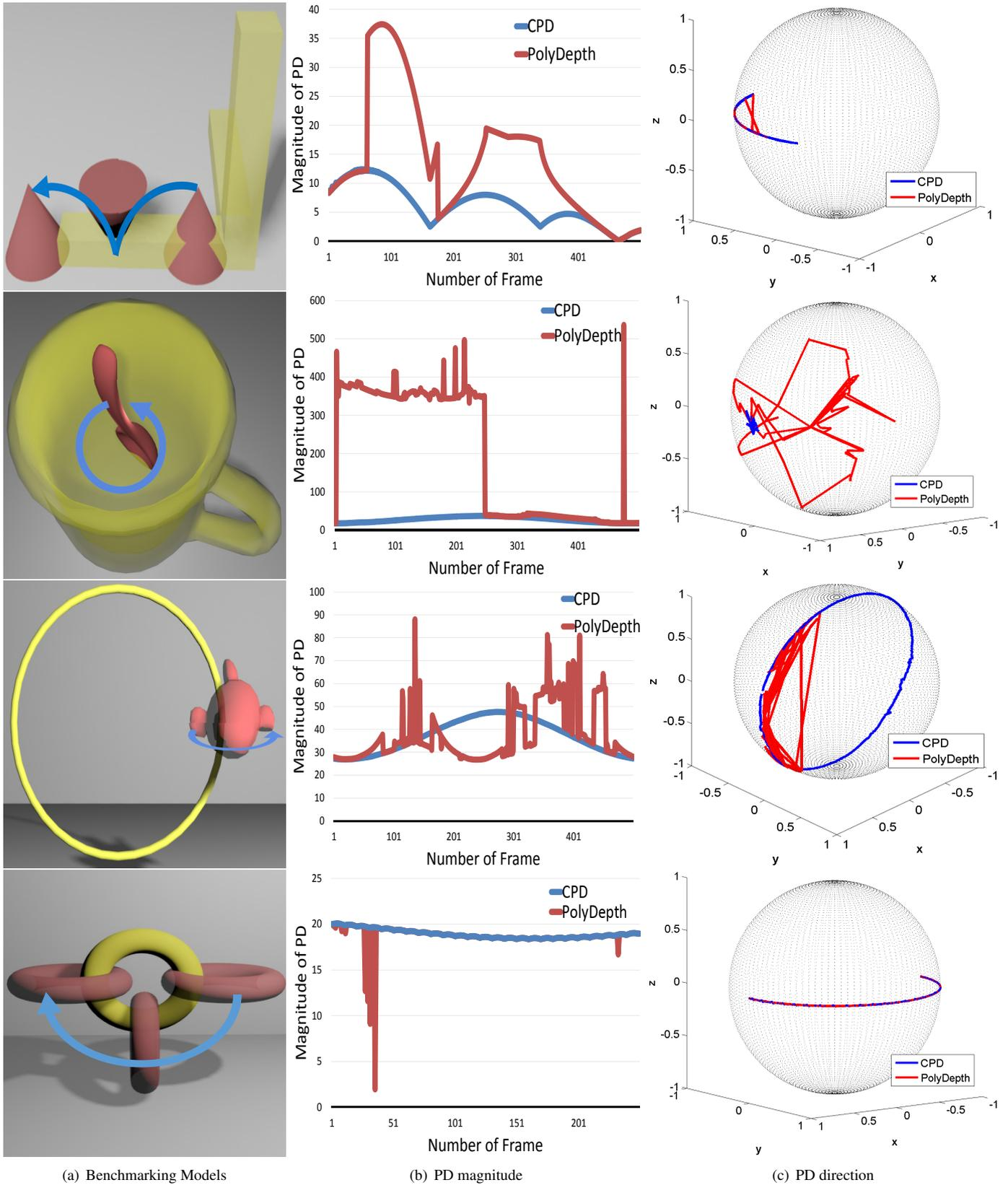
Figure 11: Various CPD benchmarks. (a) From top to bottom: cone/axes, spoon/cup, fish/torus, torus/torus. In each figure, the red model moves along the blue arrow while penetrating into the yellow model (b) PD magnitudes of our CPD and PD by PolyDepth. (c) PD directions of our CPD and PD by PolyDepth.
