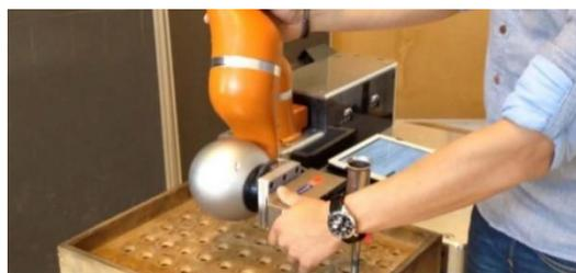
(b) An operator interacting with the robot and piloting it to a coordinate [11]
