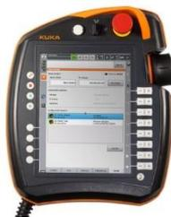
**Figure 2.** KUKA smartPAD [10]
