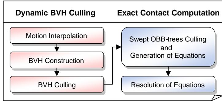
Fig. 4.1: **The two-stage pipeline of our continuous collision-detection algorithm (adapted from [60]).** The algorithm computes the time of collision and the contact location from two successive configurations of an articulated model.
