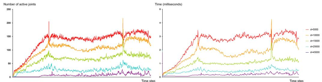
Fig. 6.5: **Performance of our algorithm depending on the viewer's distance.** Our algorithm automatically decreases the number of active joints when the distance  $d$  between the viewer and the pendulum increases (left), reducing the computational cost of the simulation (right).
