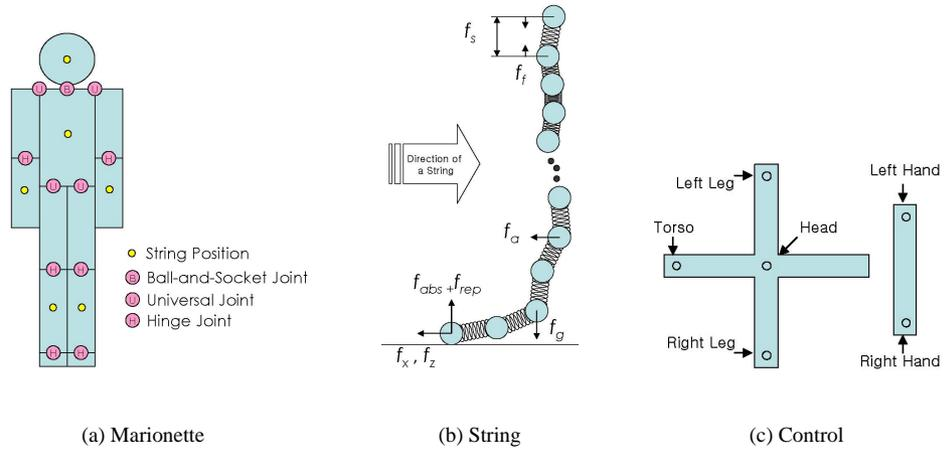
Fig. 5.1: **Modeling.** A string is modelled as a chain of particles undergoing different forces like spring force  $f_s$ , inner friction  $f_f$ , gravity  $f_g$ , air friction  $f_a$ , ground friction  $f_x, f_z$ , ground absorption  $f_{abs}$  and ground repulsion  $f_{rep}$ .
