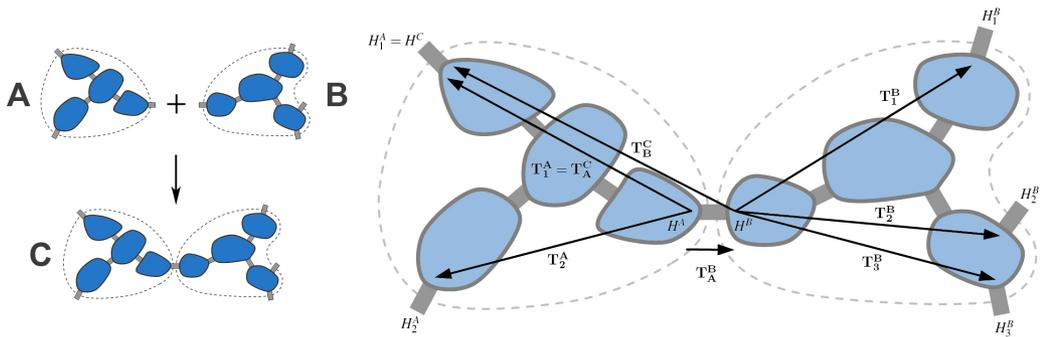
Fig. 4.2: **The kinematic representation used in our continuous collision-detection algorithm.** The figure shows the principal joint transformation  $\mathbf{T}_A^B$ , the principal-to-secondary handle transformations  $\mathbf{T}_1^A$ ,  $\mathbf{T}_2^A$ ,  $\mathbf{T}_1^B$ ,  $\mathbf{T}_2^B$  and  $\mathbf{T}_3^B$ , and the child-to-parent transformations  $\mathbf{T}_A^C$  and  $\mathbf{T}_B^C$ .
