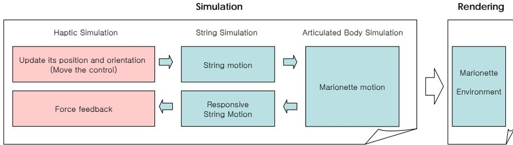
Fig. 5.4: **System Diagram.** The red block is an asynchronous process whereas the blue blocks are synchronized with each another.
