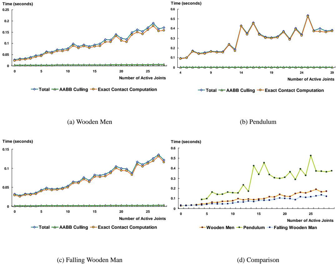
Fig. 6.7: CCD timings for three benchmarks and a comparison between them. Each graph shows a timing profile of CCD performance with AABB culling and exact contact computation steps for three benchmarking scenarios, and their comparison. The CCD time complexity gradually increases as a function of the number of active joints.
