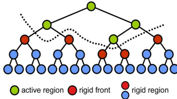
Fig. 3.2: **Assembly tree of an articulated body.** Adaptive articulated-body dynamics simulates only some of the joints in the articulated bodies, which form the active region.
