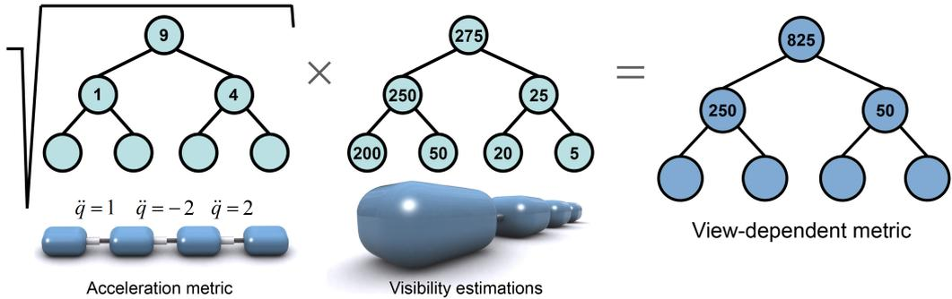
Fig. 3.3: **View-dependent motion metric.** The view-dependent motion metric is obtained by combining a priori motion metrics with visibility estimations.
