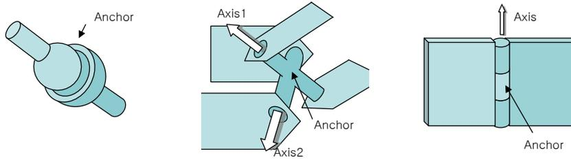
Fig. 5.2: **Different Joint Types.** *ball and socket joint, universal Joint, hinge joint (from left to right)*
