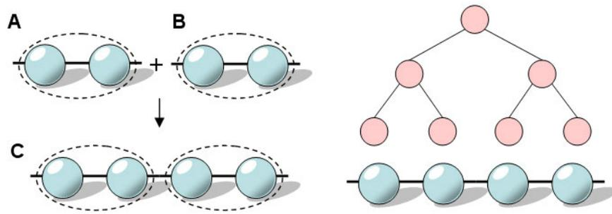
Fig. 2.1: **An example of a chain-like articulated body and its assembly tree.** *Left:* Two sub-articulated bodies A and B are attached by a joint to form a new articulated body C. *Right:* The corresponding assembly tree for the articulated body C. Here, the root node represents the articulated body C; the internal nodes represent the sub-articulated bodies A and B; the leaf nodes represent all the rigid bodies in C.
