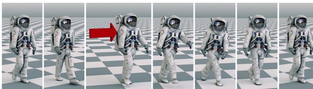
**Figure 14.** Simulated walking motion in the gravity of the Moon with external force perturbation, where the red arrow shows the direction of the external force with 75N for 0.2 sec.
