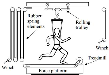
(a) Erect cable suspension system [15]
