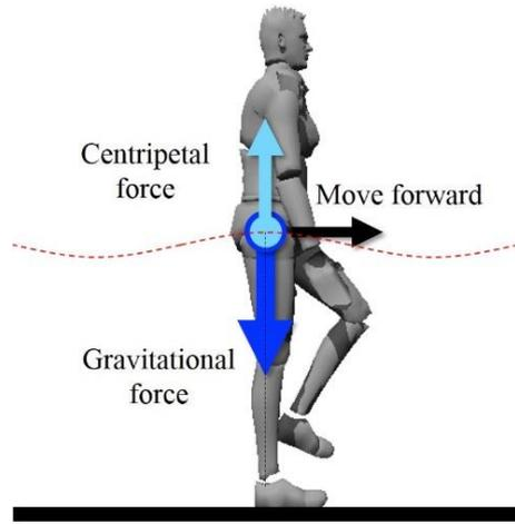
**Figure 3.** The centripetal force and gravitational force occur when a biped walks. The red dot line is a center of mass trajectory.
