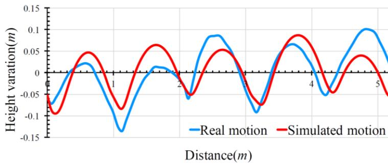
(c) The COM height variation with respect to the run distance for the real and simulated motions.
