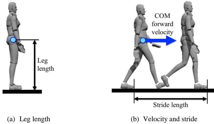
**Figure 8.** Illustrations of leg length, COM forward velocity and stride length
