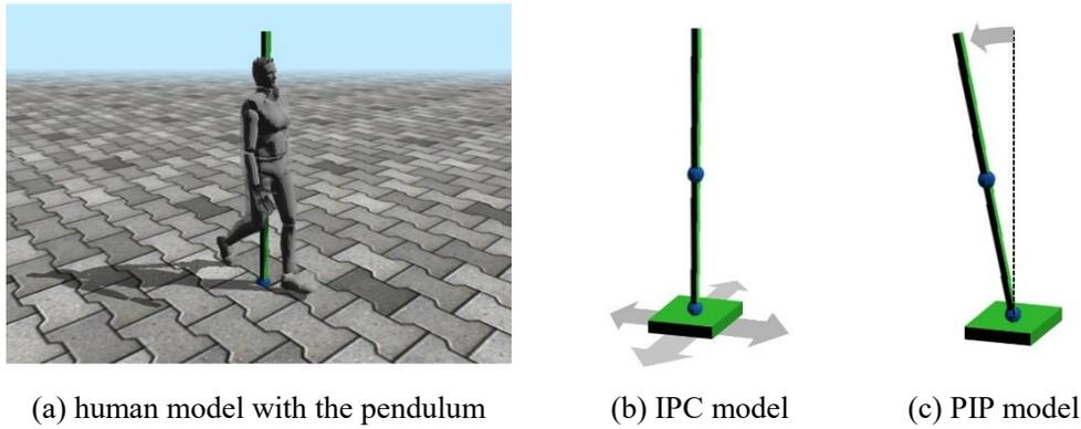
**Figure 6.** Illustrations of the human model and two types of inverted pendulum models.
