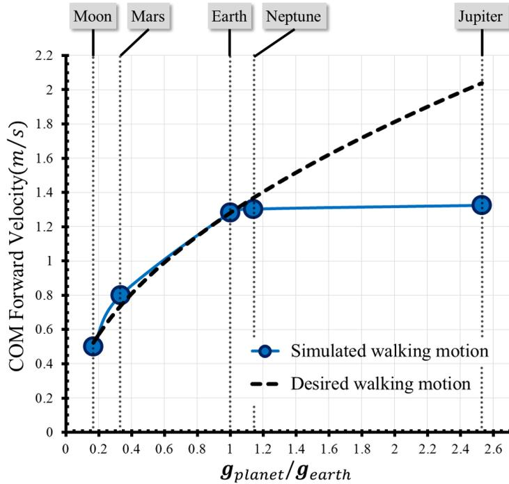
**Figure 15.** Comparison against an analytical model using Froude number for walking motion. The x and y axes in the graph denote the normalized gravity with respect to the Earth's gravity and the COM forward velocity, respectively. The dotted line denotes a curve that is based on the analytical model using Equation 3 and the blue line denotes a curve that is based on our simulation results. These curves show a similar pattern of results except for Jupiter.
